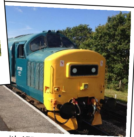
6975 , class 37, with 1750 BHP engine and weighs in at 100 tons!
